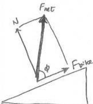
$$\begin{aligned} |F_{\text{net}}| &= \sqrt{(F_{\text{bike},x})^2 + N^2} \\ &= \underline{644.7 \text{ N}} \quad (644.7056028 \text{ N}) \end{aligned}$$
