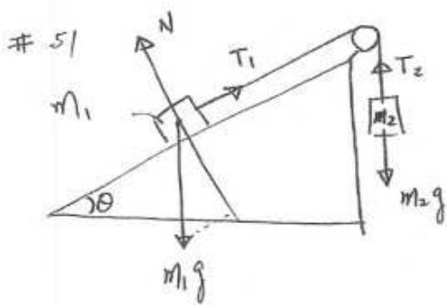
$$\begin{aligned}m_1 &= 3.70 \text{ kg} \\m_2 &= 2.30 \text{ kg} \\&\theta = 30^\circ\end{aligned}$$
