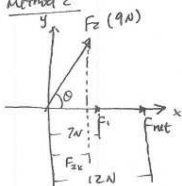
$$\begin{aligned} \sum F_x &= 12\text{N} = F_{1x} + F_{2x} \\ &= 7.0\text{N} + F_{2x} \quad \therefore \underline{\underline{F_{2x} = 5.0\text{N}}} \end{aligned}$$
