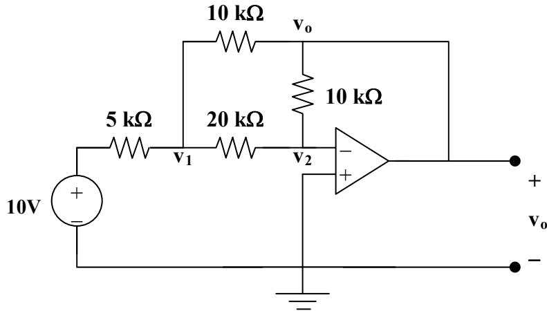
$$\text{But } v_2 = 0. \text{ Hence } 40 - 4v_1 = v_1 + 2v_1 - 2v_o \longrightarrow 40 = 7v_1 - 2v_o \quad (1)$$
