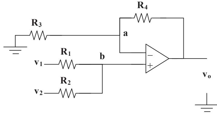
$$\text{At node } b, \frac{v_b - v_1}{R_1} + \frac{v_b - v_2}{R_2} = 0 \longrightarrow v_b = \frac{\frac{v_1}{R_1} + \frac{v_2}{R_2}}{\frac{1}{R_1} + \frac{1}{R_2}} \quad (1)$$
