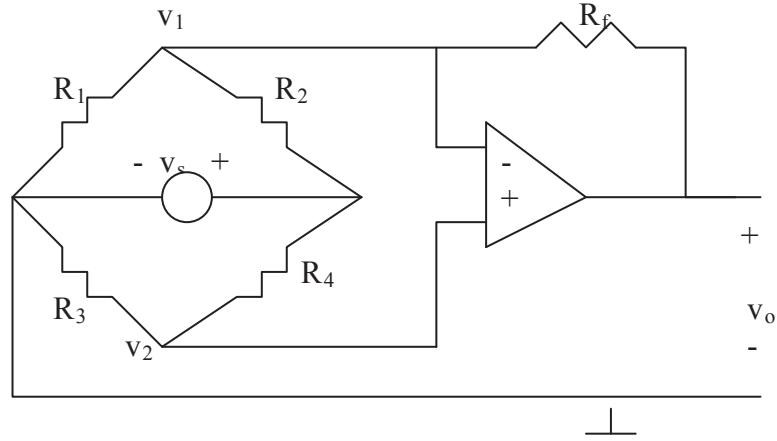
We notice that  $v_1 = v_2$ . Applying KCL at node 1 gives
